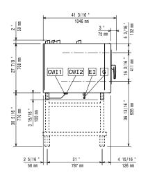
CWI1 = Cold Water inlet 1 Electrical inlet (power)
