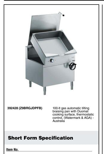
Suitable for natural gas or LPG. Burners in AISI 441 with flame failure device. Duomat cooking surface for roasting, browning, stewing, preparation of sauces, sautéing, boiling and braising. Can be installed on cantilever systems. Installation on wheels is not available. Includes mechanism to automatically tilt the pan and double-skinned lid in stainless steel. Cooking temperature can be set through thermostat and the energy input through an energy regulator.
