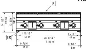
EQ = Equipotential screwG = Gas connection
