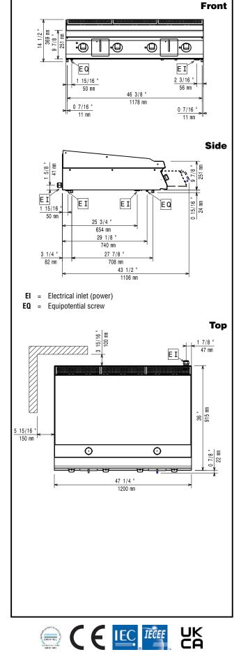
Modular Cooking Range Line EVO900 1200mm Electric Fry Top HP, Smooth and Ribbed Scratch Resistant Chromium Plate The company reserves the right to make modifications to the products without prior notice. All information correct at time of printing.
