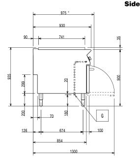
EQ = Equipotential screwG = Gas connection
