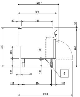
EQ = Equipotential screwG = Gas connection
