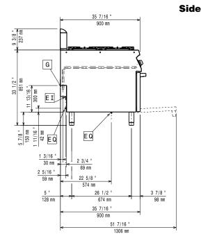
EI = Electrical inlet (power)G = Gas connection
