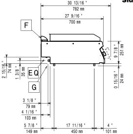
EQ = Equipotential screwG = Gas connection
