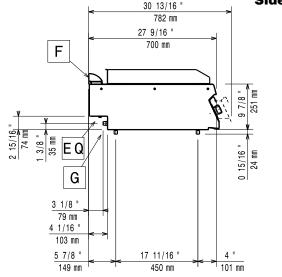
EQ = Equipotential screwG = Gas connection
