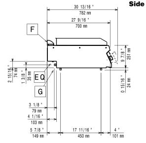
EQ = Equipotential screwG = Gas connection
