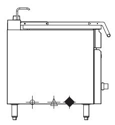
3/4" BSP Gas Inlet 10 AMP/230V Plug with 3m Lead Cable - 1/2" Quick Connect Water Inlet
