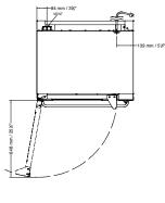
Model E31D4/2 shown Model E31D4/2C dimensions: Add 31/4" / 82mm to vertical heights
