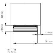
Width: 1220mm Depth: 1128mm Height: 1427mm Nett weight: 141.5kg Packed weight:
