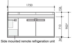
320 510 Length of multiple cabinets At each joint ±5mm -5mm to +10mm Power cord with 3-Pin plug
