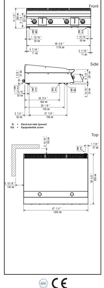
Modular Cooking Range Line 900XP 1200mm Electric Fry Top HP, Smooth scratch resistant chromium Plate The company reserves the right to make modifications to the products without prior notice. All information correct at time of printing.
