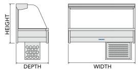
Note: For overall height dimensions, add height of motor cage (450 mm).
