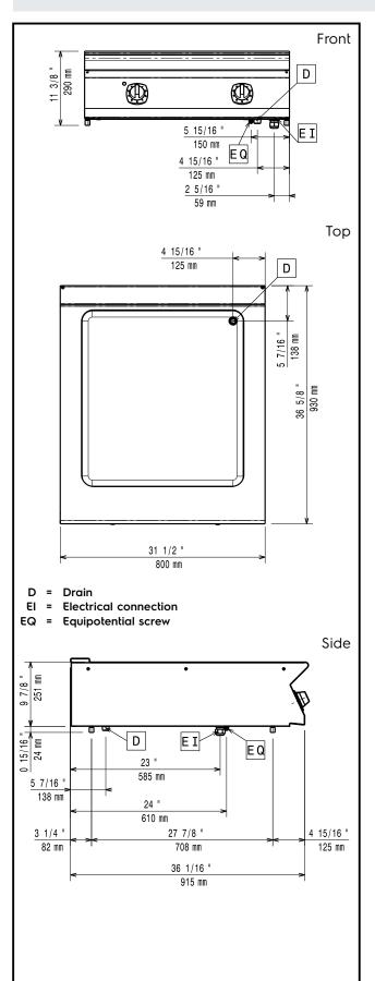
**Electric** Supply voltage: 391125 (E9BMEHB000) 400 V/2N ph/50/60 Hz Total Watts: 4.4 kW Water: Water Drain: 50 mm **Key Information:** Usable well dimensions (width): 630 mm Usable well dimensions (height): 160 mm Usable well dimensions (depth): 685 mm 30 °C MIN; 90 °C MAX
