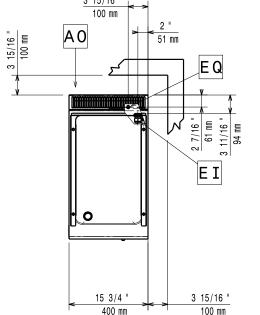
EI = Electrical connection EQ = Equipotential screw
