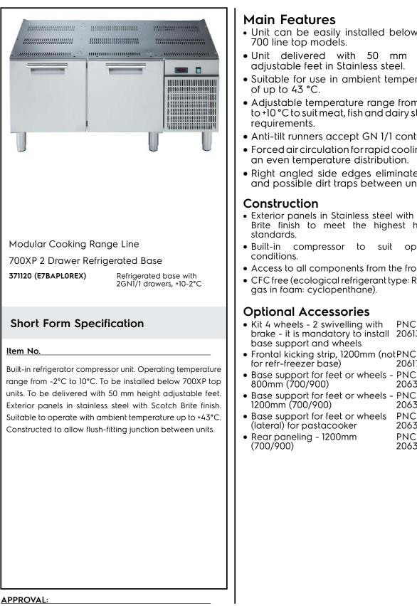
• Unit can be easily installed below other
