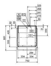
CWI = Cold Water inlet **XD** = Detergent connection D Drain XI = Chemicals inlet
